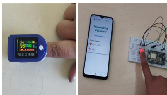
FIGURE 4 . Measurement of SpO2 and BPM Using Sensor
