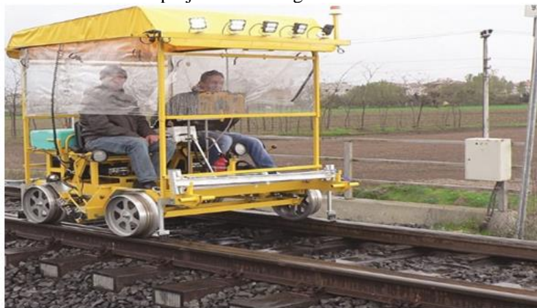
Fig.1 Crack inspection trolley
