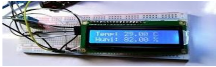
Fig: 4 Temperature and Humidity Value on LCD Display
