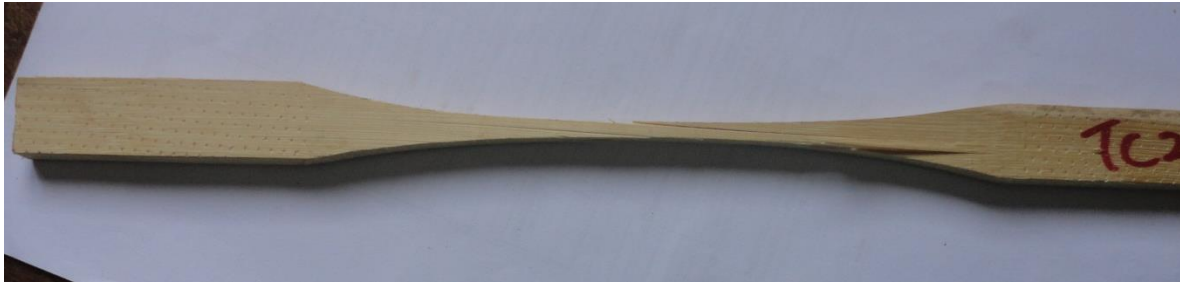
Figure 13: Tensile failure of a bamboo strip with outer skin removed
