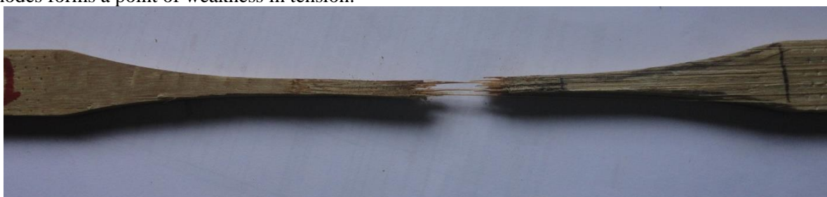
Figure 12: Tensile failure of a bamboo strip with node at the center
