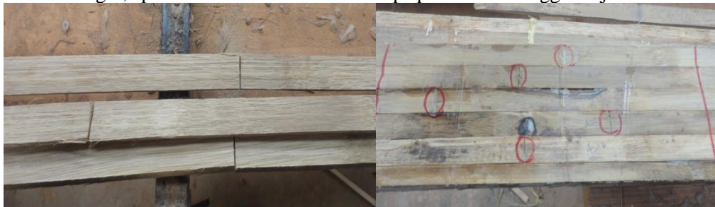
Figure 5: Bamboo Strips pieces with staggered joints
