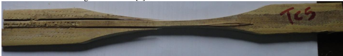
Figure 14: Tensile failure of a bamboo strip with outer skin intact and no node.
