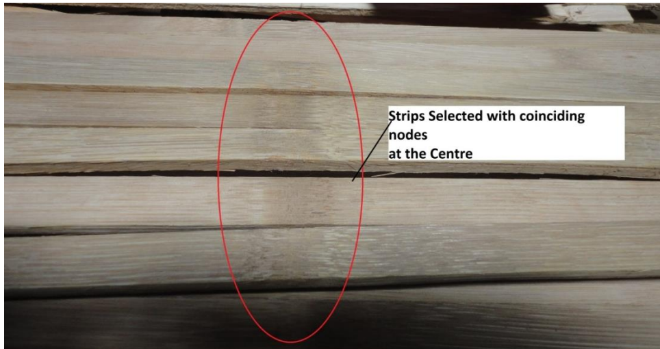
Figure 4: Bamboo Strips arranged with the nodes at the mid-point
