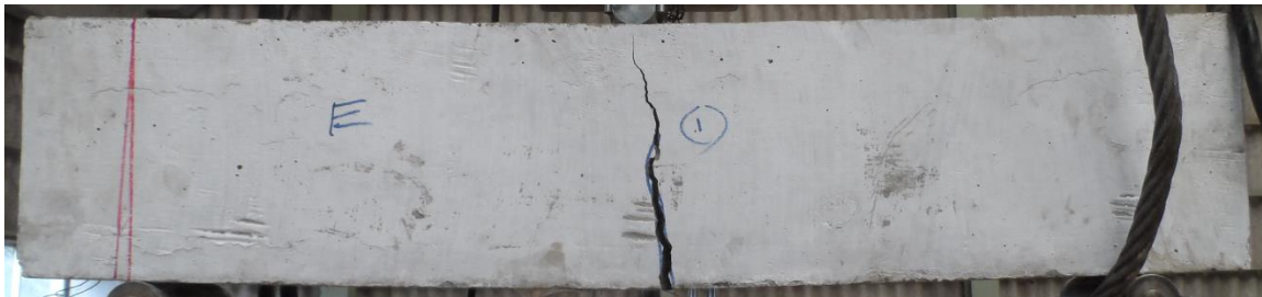
6.6 Failure Mode of BR4MPΦ20
