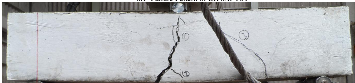
6.2 Failure Pattern of BR4MPΦ25
