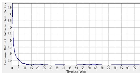
**Figure 2:** The plot of AMI versus time-delay that gives the suitable time-delay for the reconstruction of the phase space plot.
