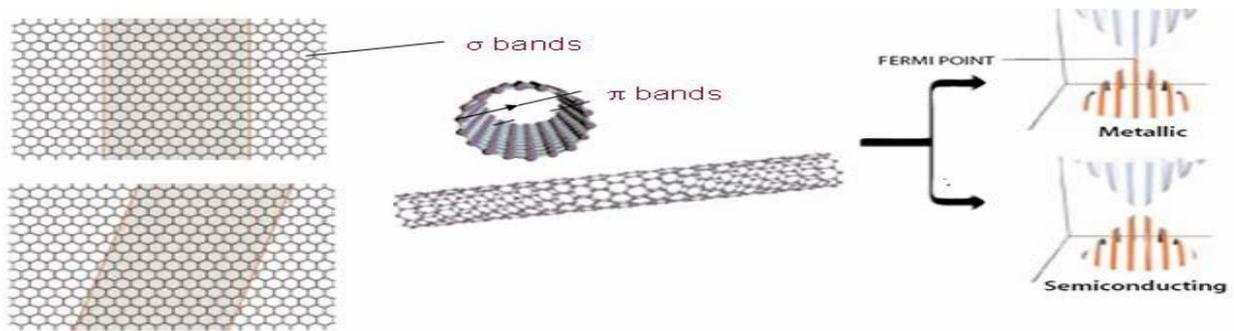
Figure 1. Carbon nano-tube at conducting stages
