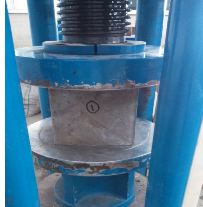
Figure 4. Testing of concrete cube
