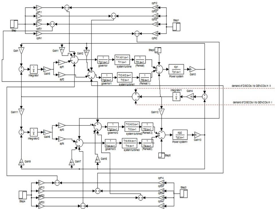
Fig. 3 MATLAB Simulation model of a Two Area power system with reheat system
