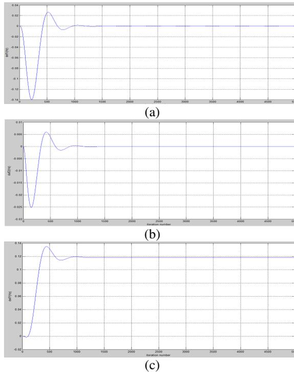
Fig.8 (a) frequency deviation in area 1,(b) frequency deviation in area 2, (c) deviation in tie-line power, for case 2 with reheat type system.
