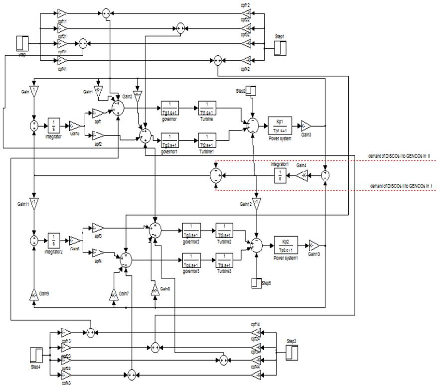
Fig. 2 MATLAB Simulation model of a two area power system with non-reheat turbine [9].
