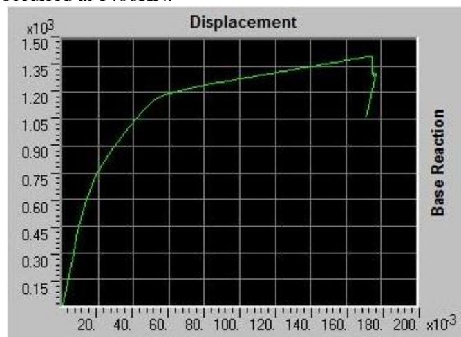
Fig.2 Non-ductile detailing load versus displacement curve
