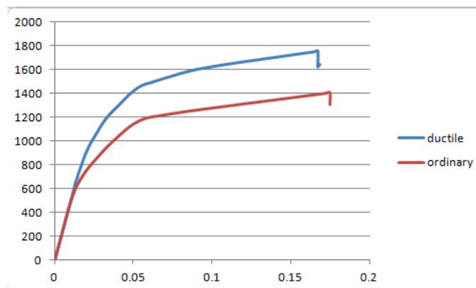
Fig.4. load versus displacement curve for Ductile and Ordinary frames
