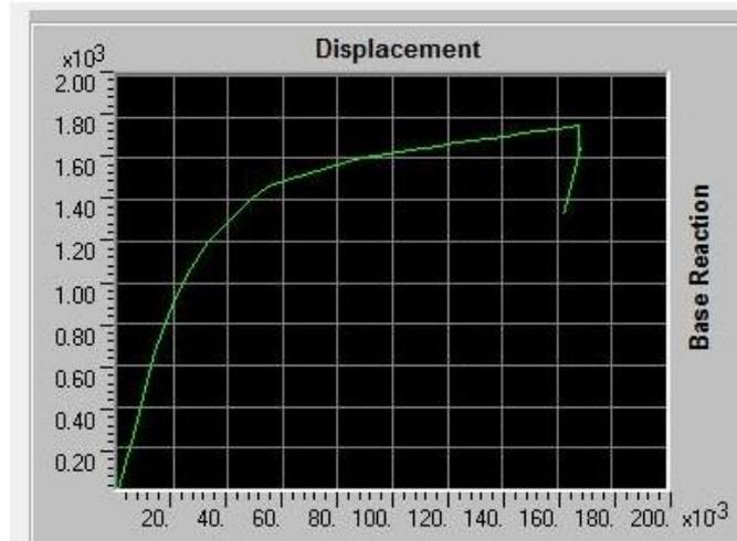
Fig.3. Ductile detailing load versus displacement curve
