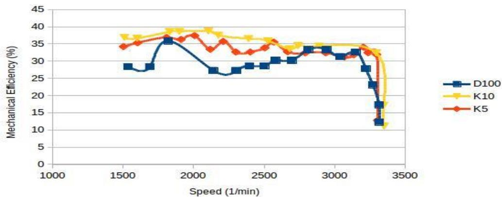
Figure 5: Mechanical Efficiency versus Speed
