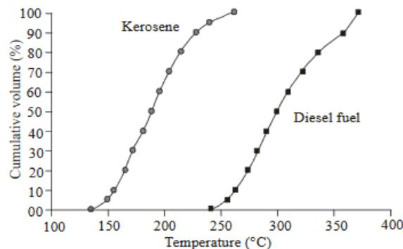
**Figure 1:** Boiling range curves of kerosene and Diesel [9]
