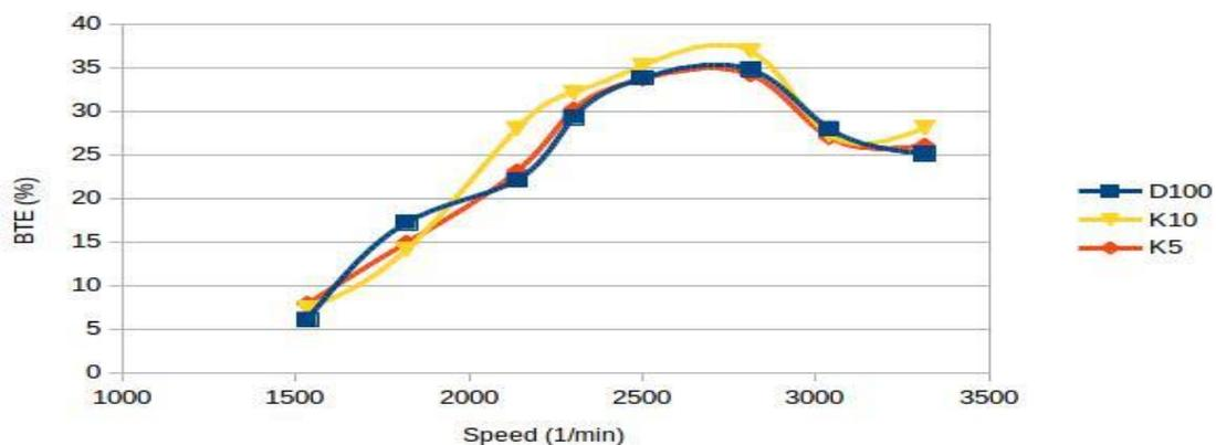
Figure 3. Brake Thermal efficiency versus speed
