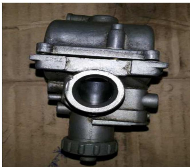
Fig. 1: (c) TVS Max 100 carburetor used
