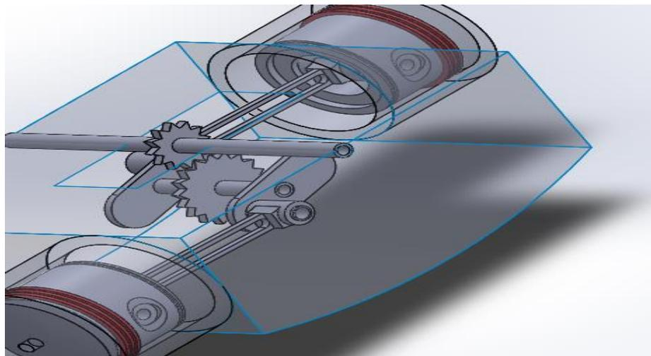
Fig. 1: (d) Introducing a Simple Gear Train in FA-300 Twin Cylinder four-stroke boxer engine
