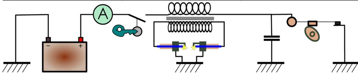
Fig. 1: (a) Ignition System of Twin-Flat Engine
