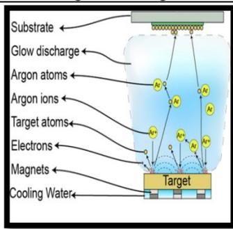
Figure 1. DC Magnetron Sputtering Technique
