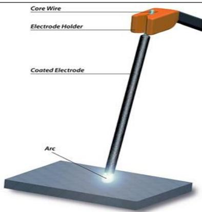
Figure 3. Hardfacing
