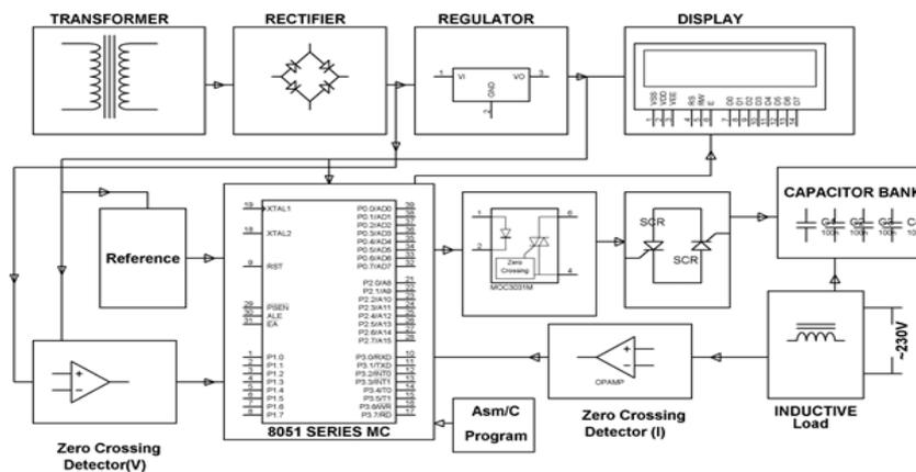
**Fig 1:** Block diagram of reactive power compensation technique
