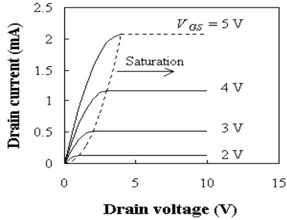
Figure 1: Typical Drain Characteristics of FET
