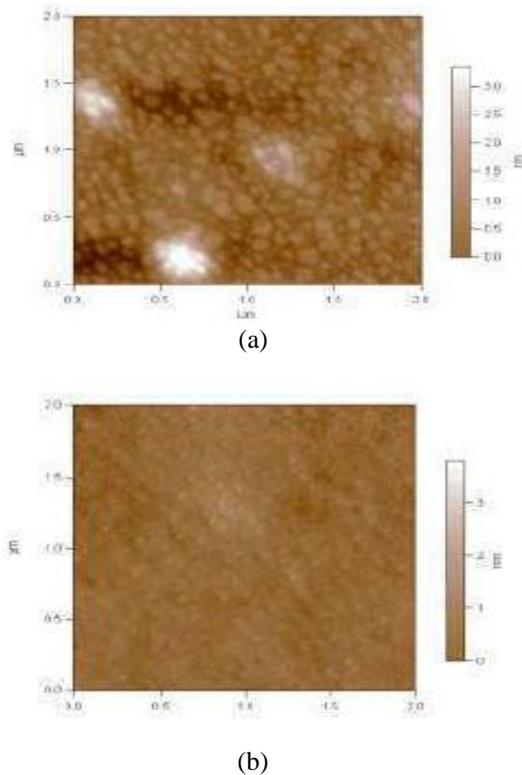
**Figure 10:** AFM images of aluminum selenide thin film (a) room temperature (b) 100°C annealing
