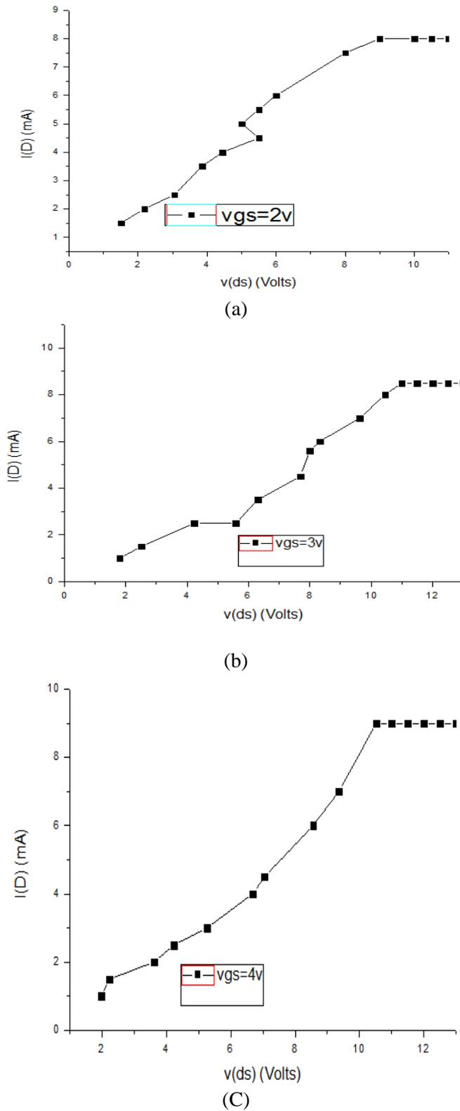
**Figure 5:** Graph between drain current and drain voltage at (a)  $V_{GS} = 2V$  (b)  $V_{GS} = 3V$  (c)  $V_{GS} = 4V$  as the Drain characteristics of MESFET using Copper as Metal contact
