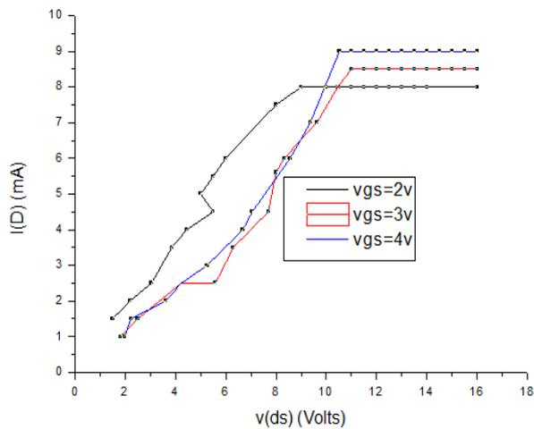
**Figure 4:** Graph between drain current and drain voltage as the Drain characteristics of MESFET using Copper as Metal contact
