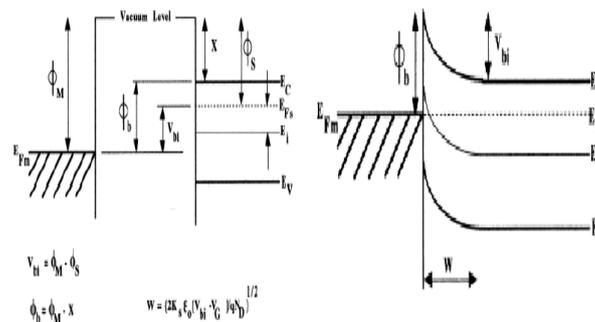
**Fig.6** The energy band diagram of Schottky contact
