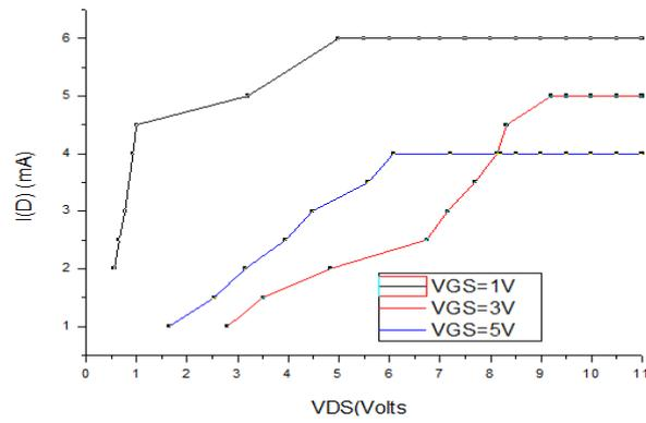
Figure 2: Graph between drain current and drain voltage as the Drain characteristics of MESFET using Aluminum
