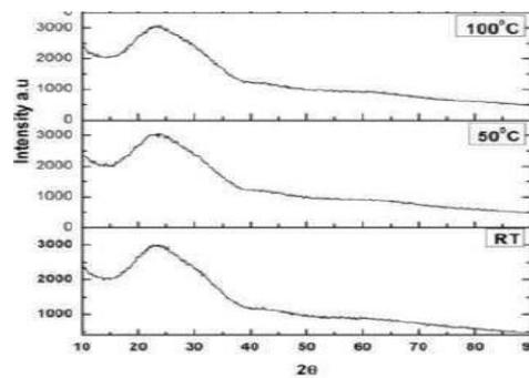
Figure 8: XRD for aluminum selenide thin films prepared at RT, Annealed at 50°C, 100°C
