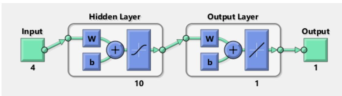
Figure 3: Block diagram of Neural network model
