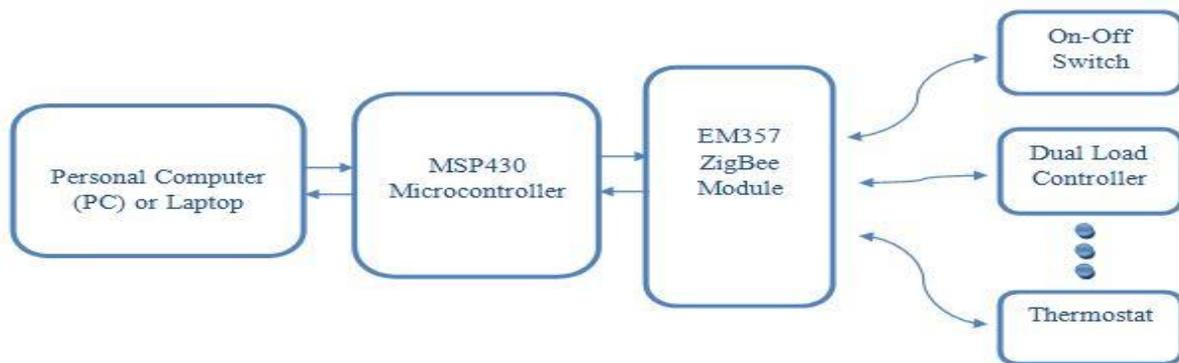
Figure 1. Block diagram of system with ZigBee Home Automation 1.2 profile supported third party devices
