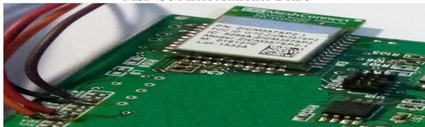
ZigBee Module Board
