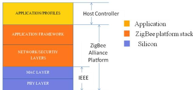
Figure 5. ZigBee Protocol Stack
