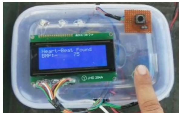
**Fig 5:** Health Monitoring unit of the device
