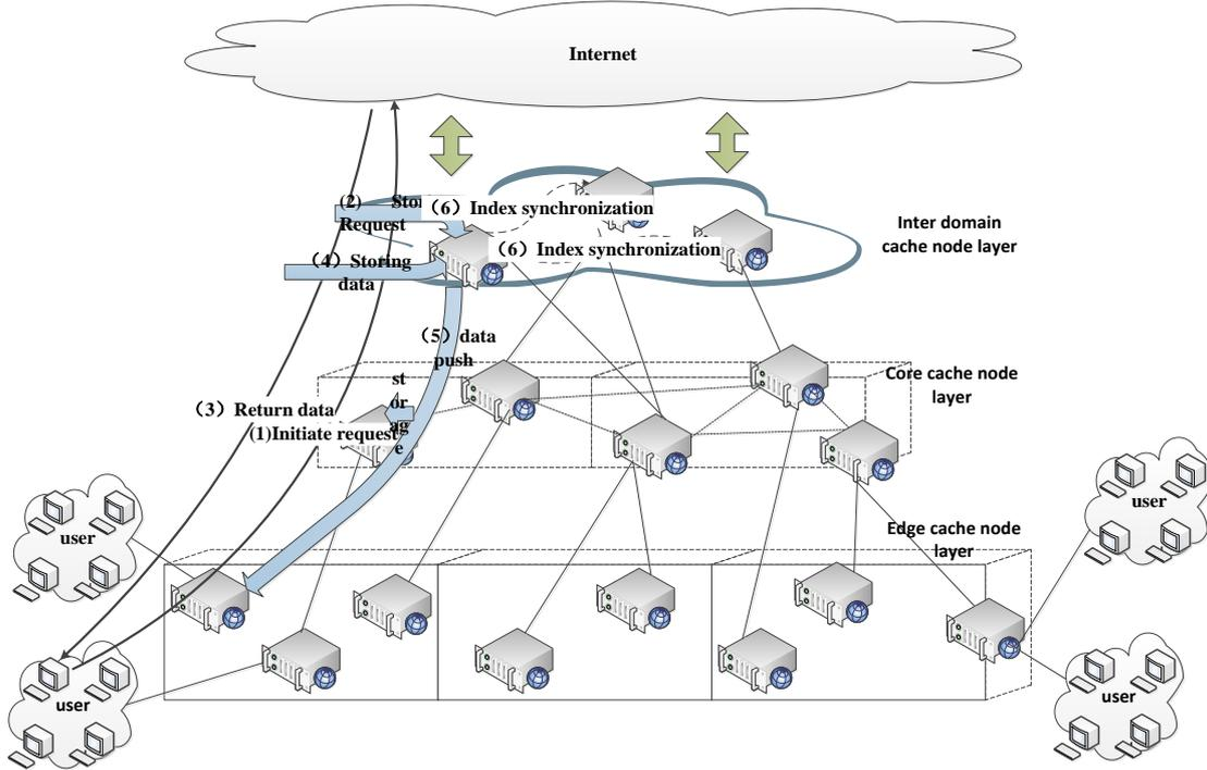
Fig. 2 The data flow of system
