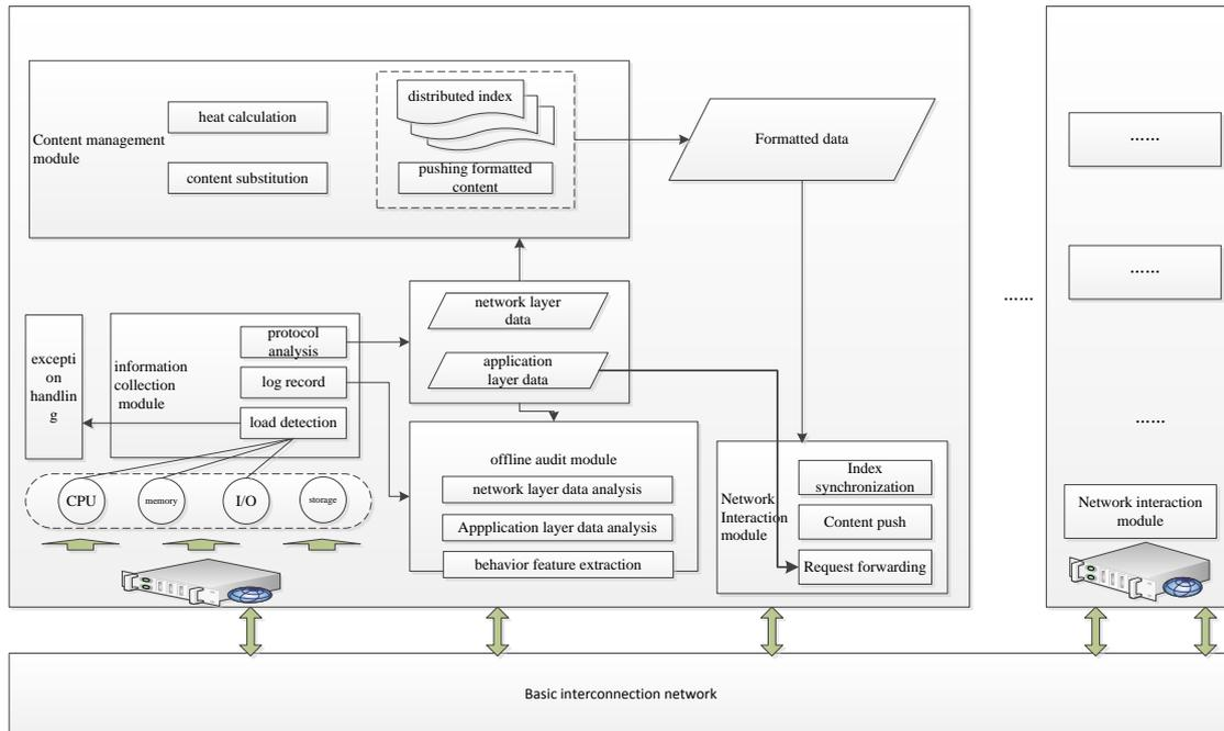
**Fig.1** The framework of merged content delivery system
