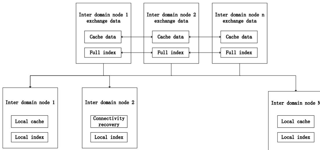
**Fig.9** The mechanism of node interaction
