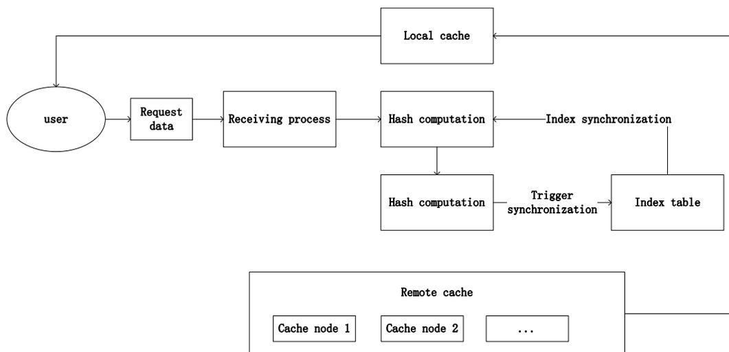
Fig.7 The work procedure of remote cache
