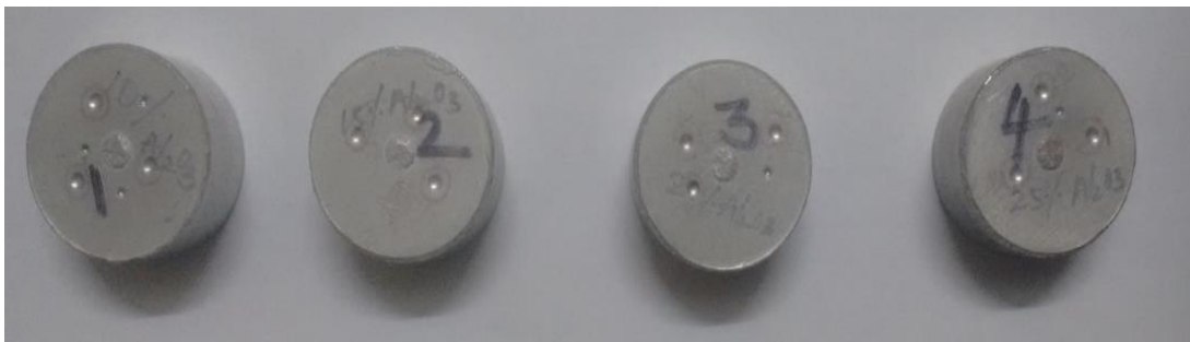
Figure 5. Samples after hardness test
