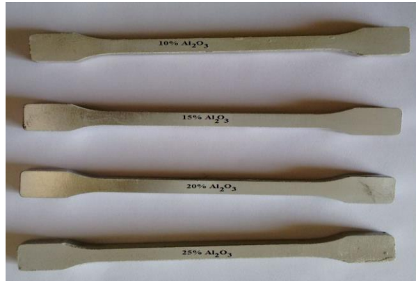
Figure 7. Specimens for tensile test
