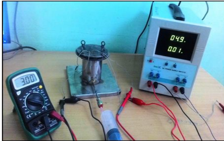
Fig. 1.2. Experimental arrangement of Wireless Sensor Node for LPG leakage measurement.
