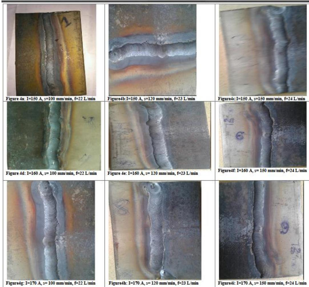
**Figure 4:** Butt joints welded at different process parameters, I is welding current, s is welding speed, f is gas flow rat
