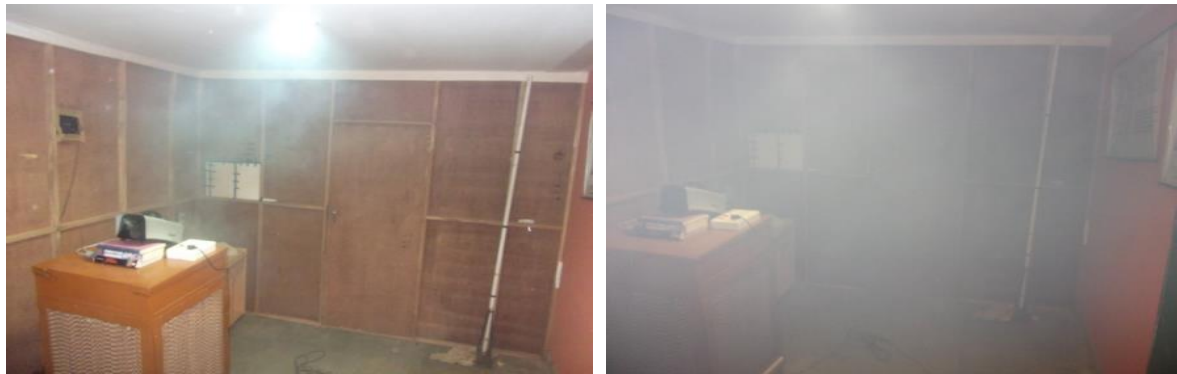
Figure 13. Actual flow patterns recorded in AC2 position by Fog machine
