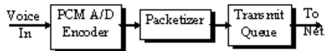
Figure 5 Block Diagram of a Station which Encodes and Sends a Voice Stream.
