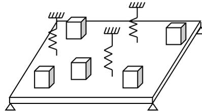
Figure1. Plate Showing Loaded Mass and Spring Uncertainty
