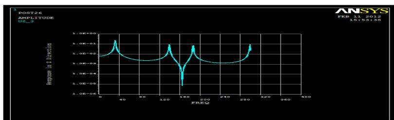
Figure 7. FRF on Log Scale at Node 3
