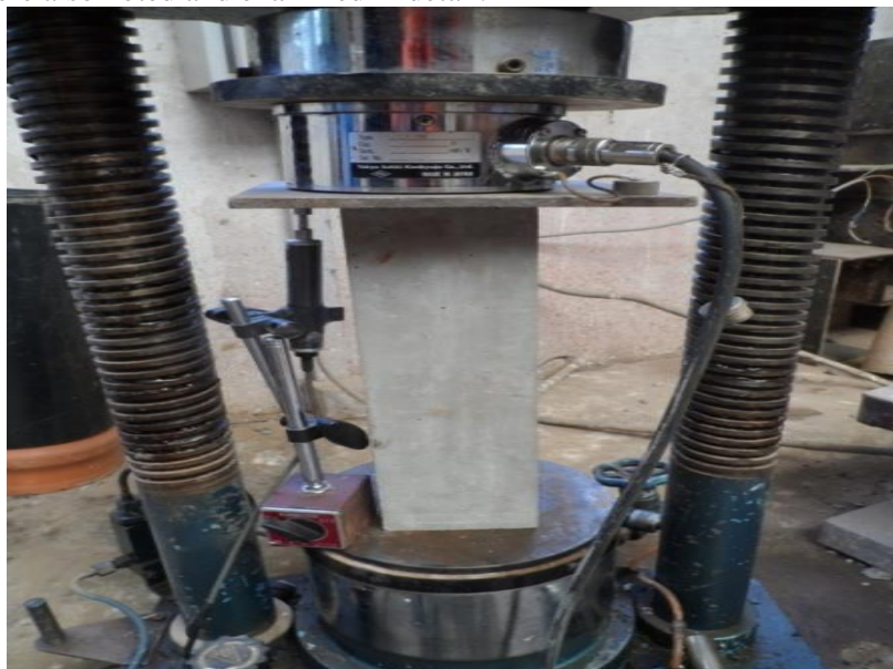
Figure 2: Test set-up of column specimen subjected to axial load
