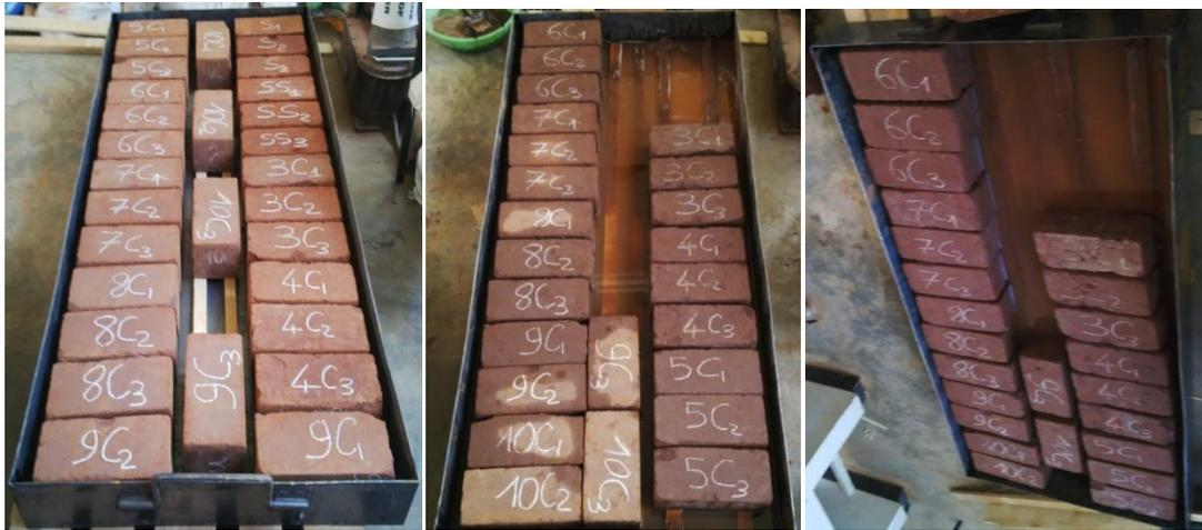
Figure 1: Illustration of Water Absorption test by Capillarity of specimens
