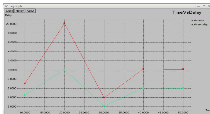
Fig 5 Comparison of AODV and AODV-SEC normalized end to end delay
