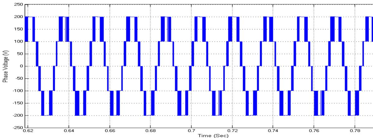
Fig.8. MLI Phase voltage
