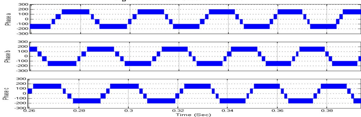
Fig.15. Five Level Output Voltages with phase shifted PWM modulation technique
