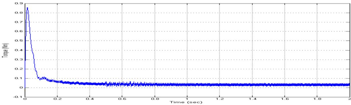
Fig.13. Electro Magnetic Torque of 5-level CHB inverter fed BLDC motor
