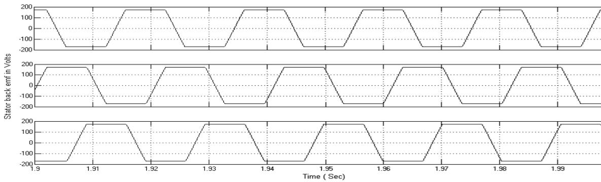
Fig.14. Three Phase Stator Back-EMFs
