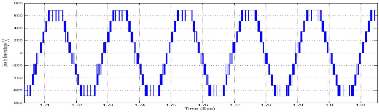
Fig. 9. Output Nine level Line to line voltage
