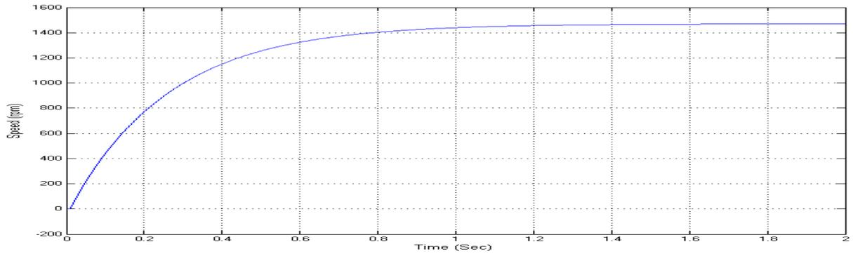
Fig.12. Output Speed of 5-level CHB inverter fed BLDC motor
