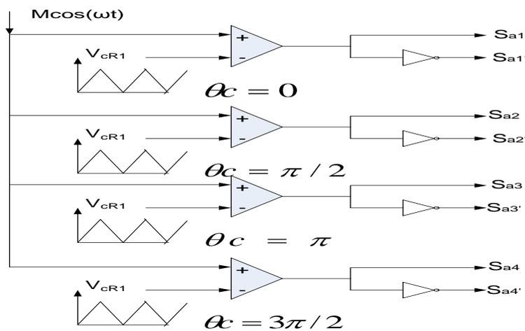
**Fig.5.** Modulation schematic
