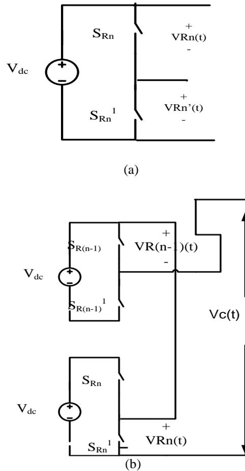
Fig. 2. (a) Isolated dc voltage source connected to inverter leg.
