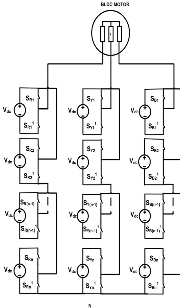
Fig.1. Proposed Multilevel inverter fed BLDC Drive
