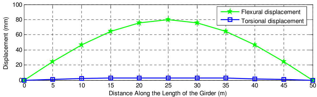
Fig. 3 Variation of flexural and torsional displacements along the length of the girder
