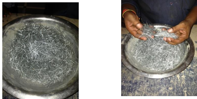
Pictures showing the steel fibers samples
