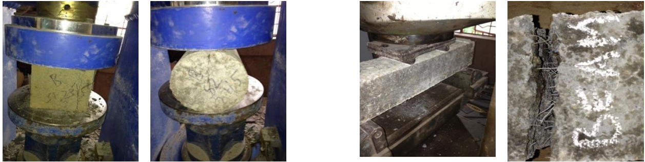
Picture showing the test method for the compressive, split tensile and flexural strengths and failure beam sample.
